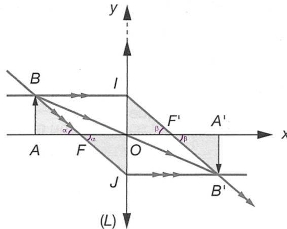
$$\tan(\alpha) = \frac{\overline{AB}}{\overline{AF}} = \frac{\overline{JO}}{\overline{FO}} \Leftrightarrow \frac{\overline{AB}}{\overline{AF}} = \frac{\overline{B'A'}}{\overline{FO}} \Leftrightarrow \gamma = \frac{\overline{A'B'}}{\overline{AB}} = \frac{\overline{FO}}{\overline{FA}}$$
