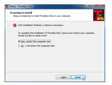
After NI-VISA Installation, the computer must be restarted. After reboot, the setup wizard restarts automatically and continues to install further software components:
