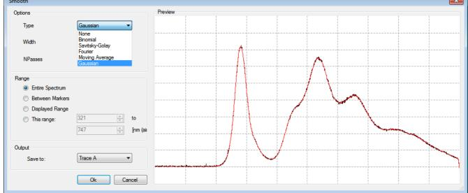
The trace to operate on is displayed in black in this dialog and the smoothed spectrum is displayed in red. Beside the displayed by default Gaussian smoothing, there are available a number of alternative smoothing methods.
