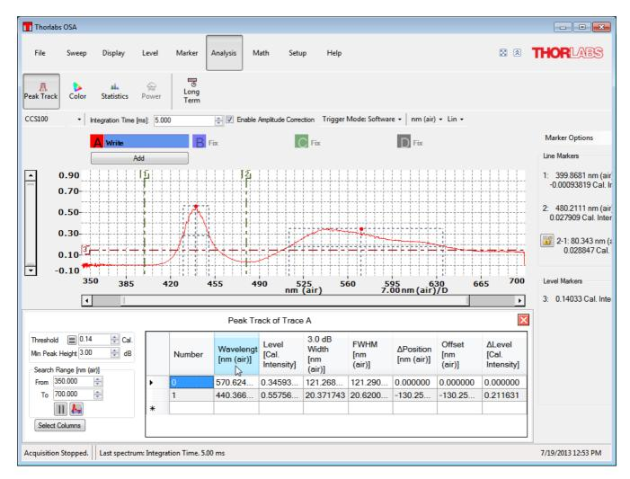
In **Peak Track** analysis mode, the position, amplitude, and width of peaks in the spectrum can be tracked over time.
